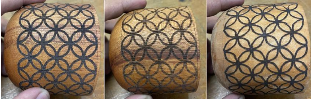
Figure 5. Batik Engraving Test on Wooden Cylinder
