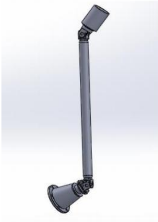
Gambar 3 Gambar 3D Propeller Shaft
