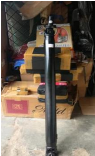
Gambar 4 Gambar Propeller Shaft
